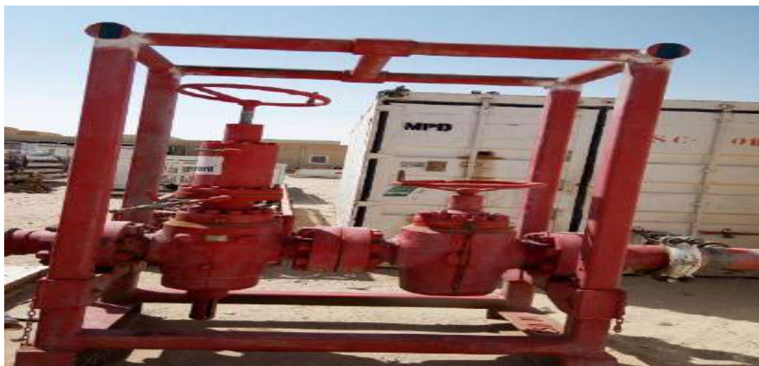
Fig II,16 : Emergency schut Down ESD
