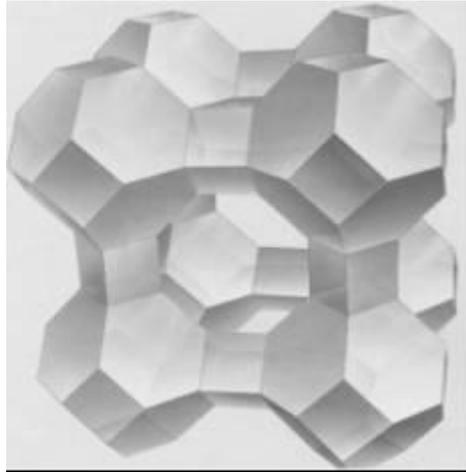
**Figure (I.1):zéolithe de type A. [DE SCAMPS, (2004)]**
