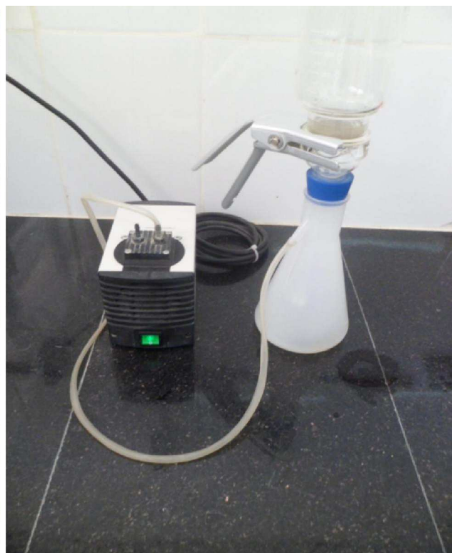
Figure 8: montage de filtration.
