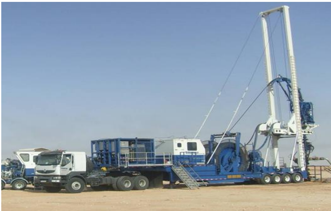
Figure.II.13. opération de coiled tubing
