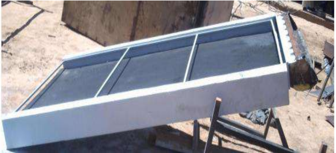
Figure 3. 2: Solar air collector made by laboratory L.E.N.R.E.Z.A [43]
