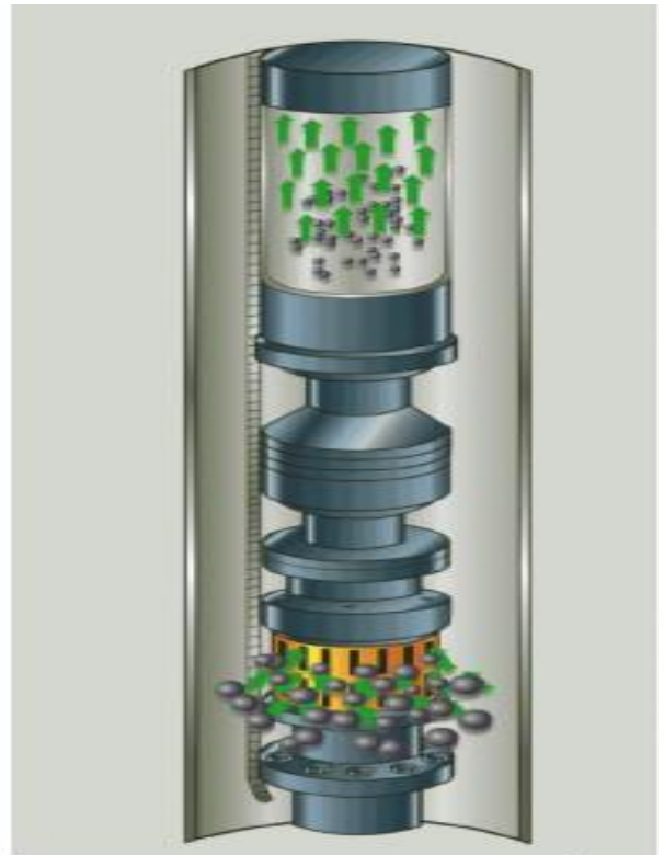
Figure II.14 Poseidon SLB gas handler (3)
