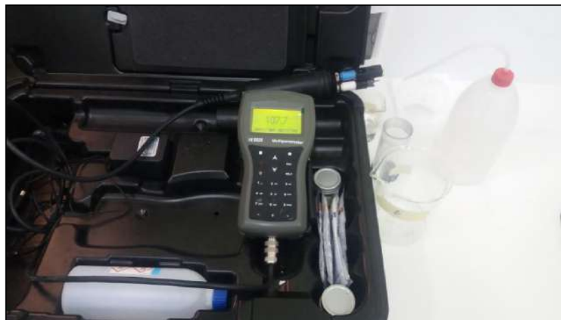
Figure III.9 : HANNA Multiparameter < HI 9829 >
