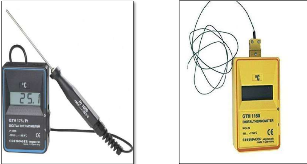
Figure.III.6 : respectivement (Thermometer Greisinger GTH 175/PT -199.9 up to +199.9 °C Sensor, TemperaturGTH 1150 C-50 bis + 1150 °C Type-K)
