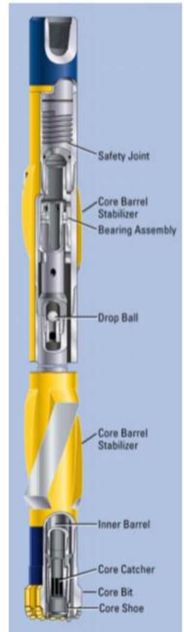
Figure 42 : 250P Core Barrel BHI (Christensen)
