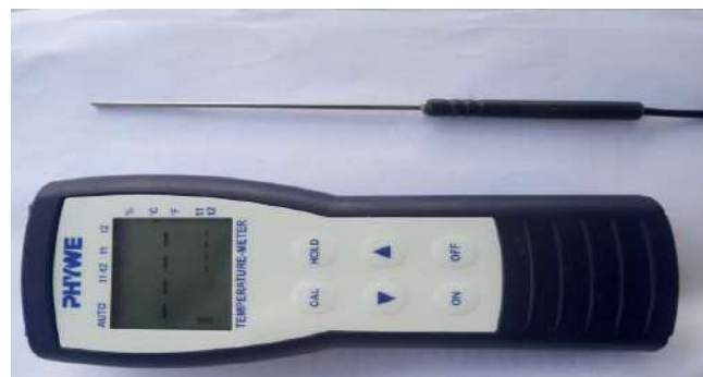
Figure II.8 : Appareil type PHYW Testo 445.
