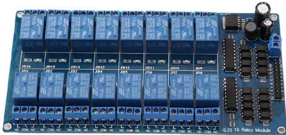
Figure III. 11: Module de 16 relais
