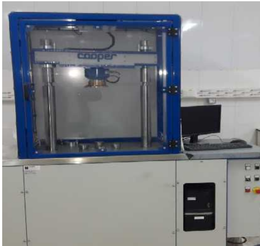
Photo II.4. Machine de compression.
