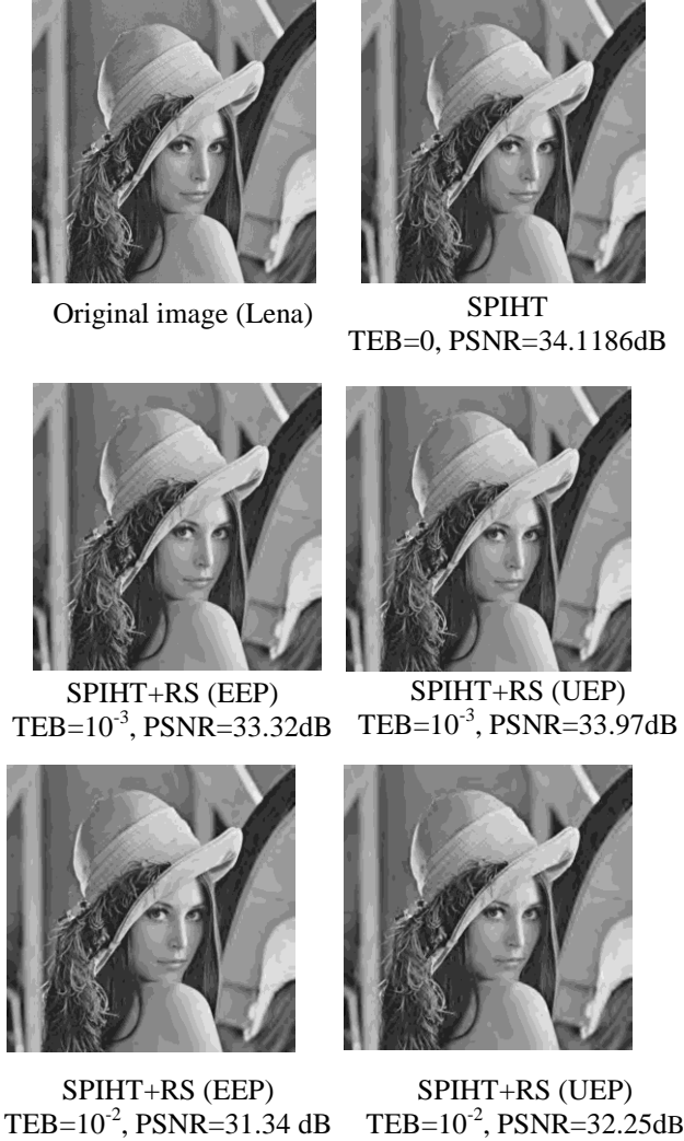
Fig. 4. Recived image (Lena) with EEP and UEP protection transmitted in BSC channel (CR = 0.25 bpp).
