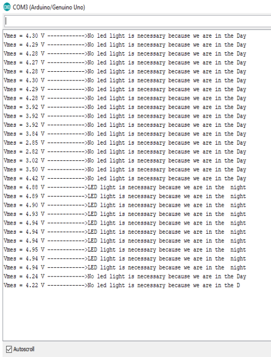
Figure 05: the variation of the measured voltage according to the intensity of the light captured
