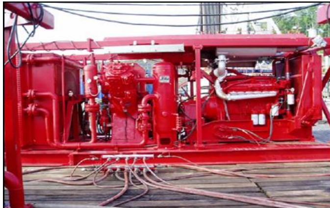
Fig.I.7. Low pressure booster
