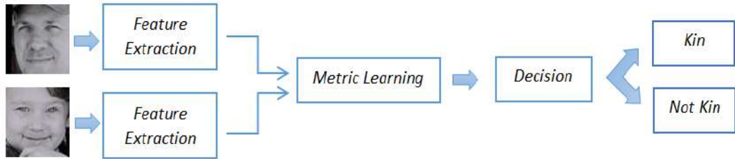
Figure 3.11: Kinship verification flowchart based on Metric classifier.
