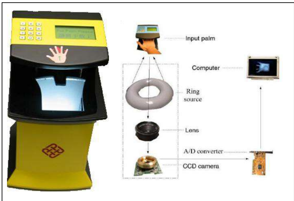
Figure III. 3: The structure of the palmprint image acquisition device.
