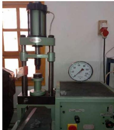
Photo 06: Essai de compression.
