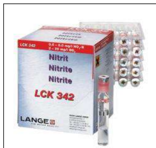
Figure V.27: Nitrite cuvette test 0.6-6.0 mg/L NO 2 -N
