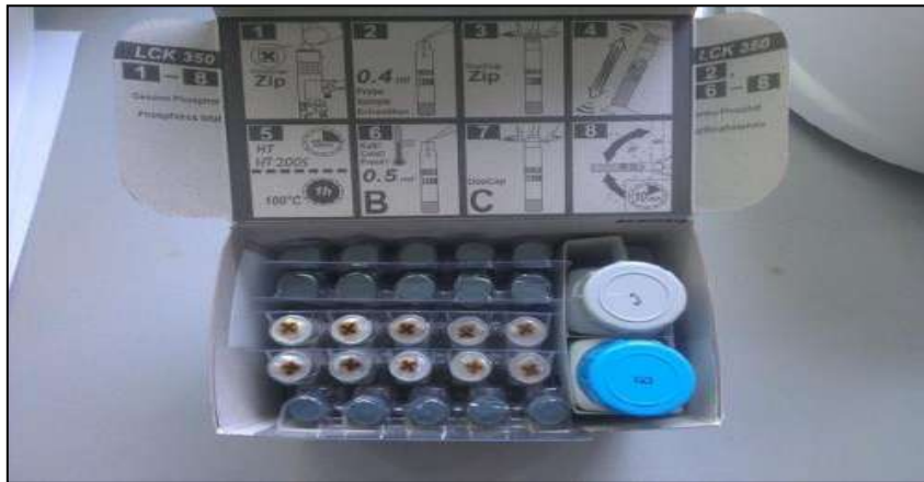
Figure V.20:phosphate (ortho/total) cuvette test 2.0-20.0 mg/l \text{PO}_4\text{-P}
