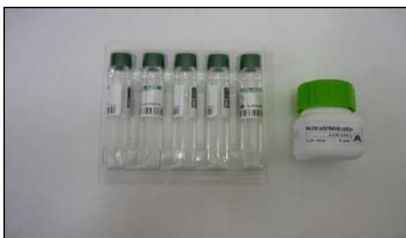
Figure V.23 : nitrate cuvette test 0.23-13.5mg/l NO 3 -N
