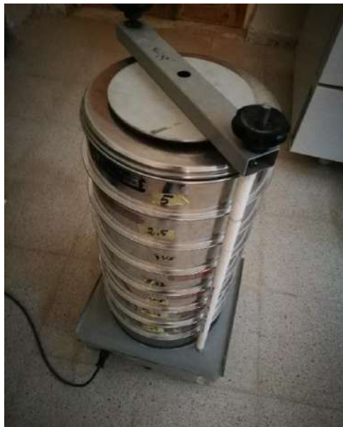
Figure II.2: particle size analysis sieves for sand.
