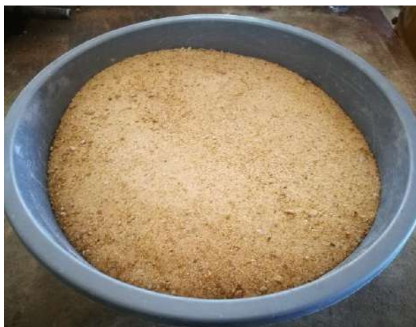
Figure I.3 fine aggregate (sand)
