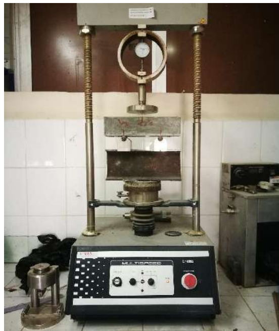
Figure II.7: Flexural strength machine
