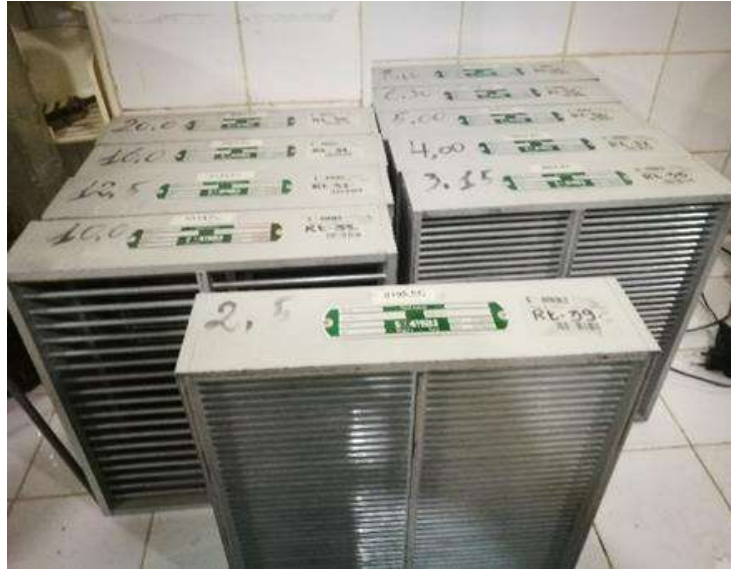
Figure II.3: Grid Sieves for gravel
