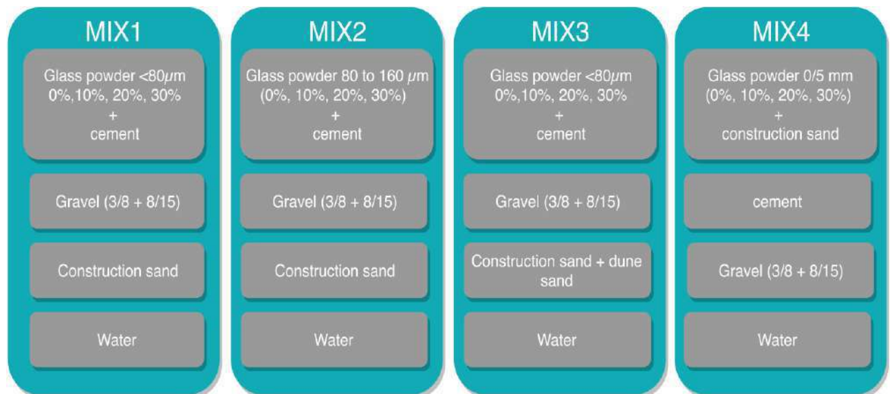
Figure II.5: compositions of the concrete mixtures
