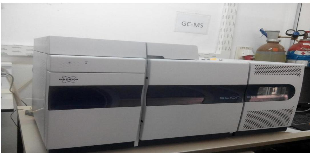
Figure (III.4): Appareil GC / MS
