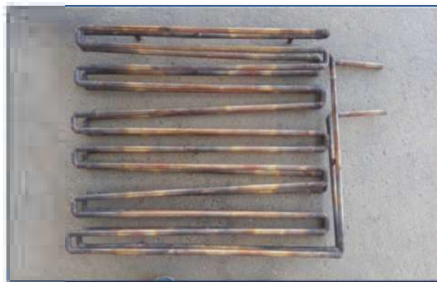
Fig II.1 Picture of the heat exchanger.
