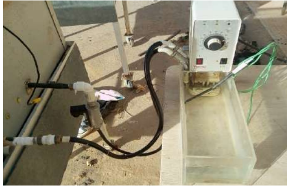
Fig II.3 Picture of the hot water source device.
