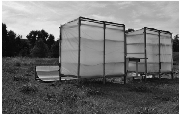
Fig I.11 Dryer 2 (left) is exposed to the concave solar concentrator. Dryer 1 (right) is the control [38].
