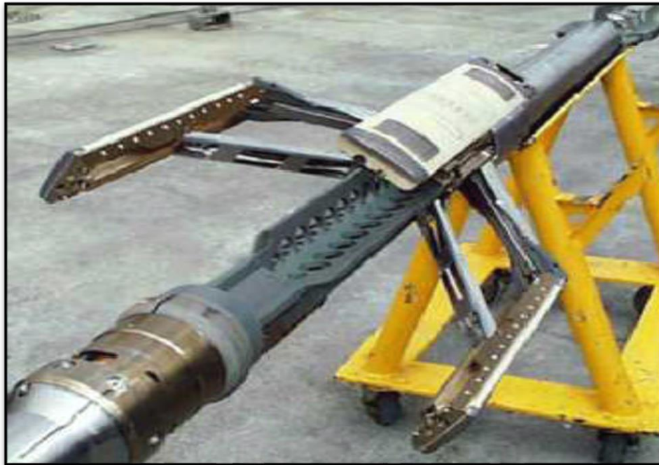
Figure. III. 5. L'outil OBMI (OIL-BASE MICRO IMAGER) (SH/DP/HMD 2019).
