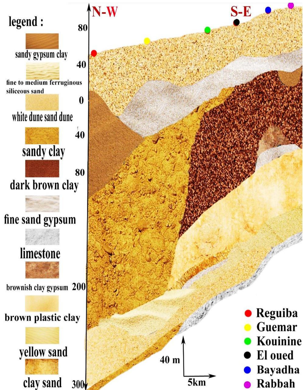
Figure (05): Geological section N ° 2, Extracted from the lithological logs of the boreholes,
