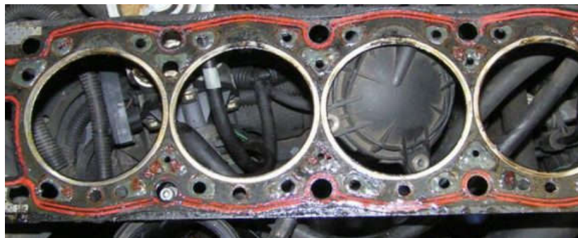
Figure II.6 joint culasse endommagé.
