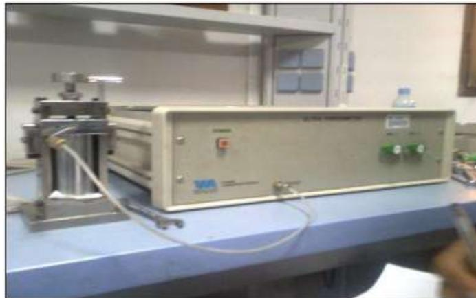
Fig 6: Mesure du volume solide [2]
