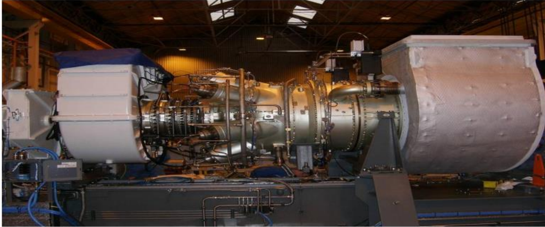
Figure II.2 : Turbine à gaz SGT-400.[2]
