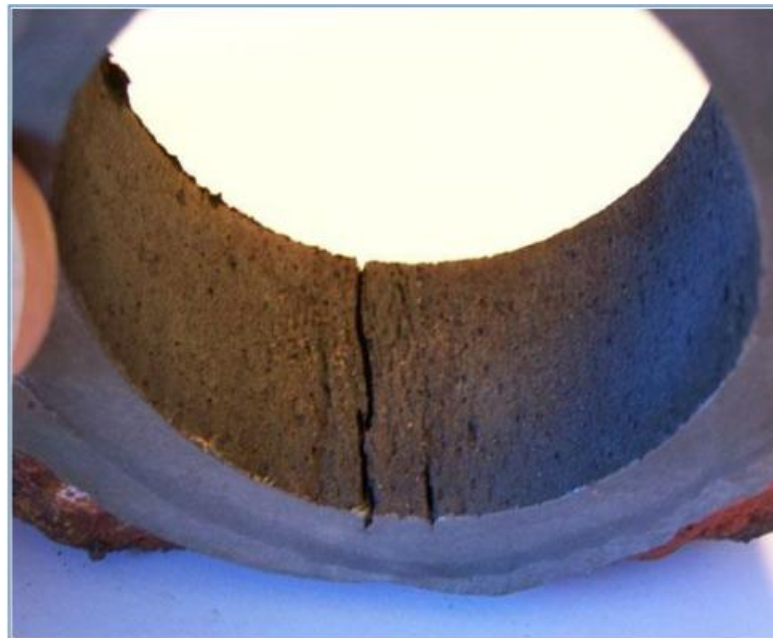
Figure I. 9. La corrosion fatigue.
