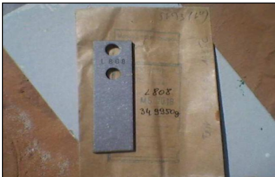
Figure 40: coupon de corrosion
