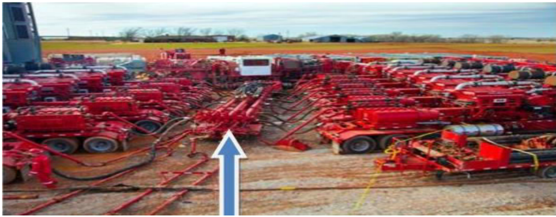
Figure III.6: Manifold de haute pression
