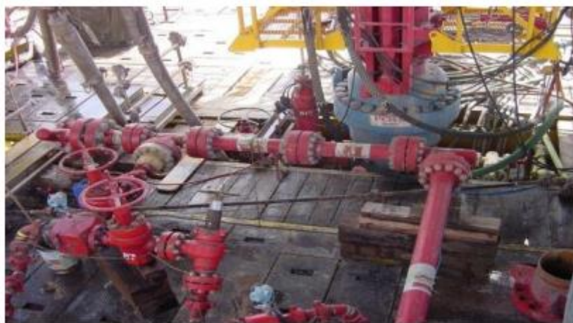
Figure II-14: Flow line Principale.
