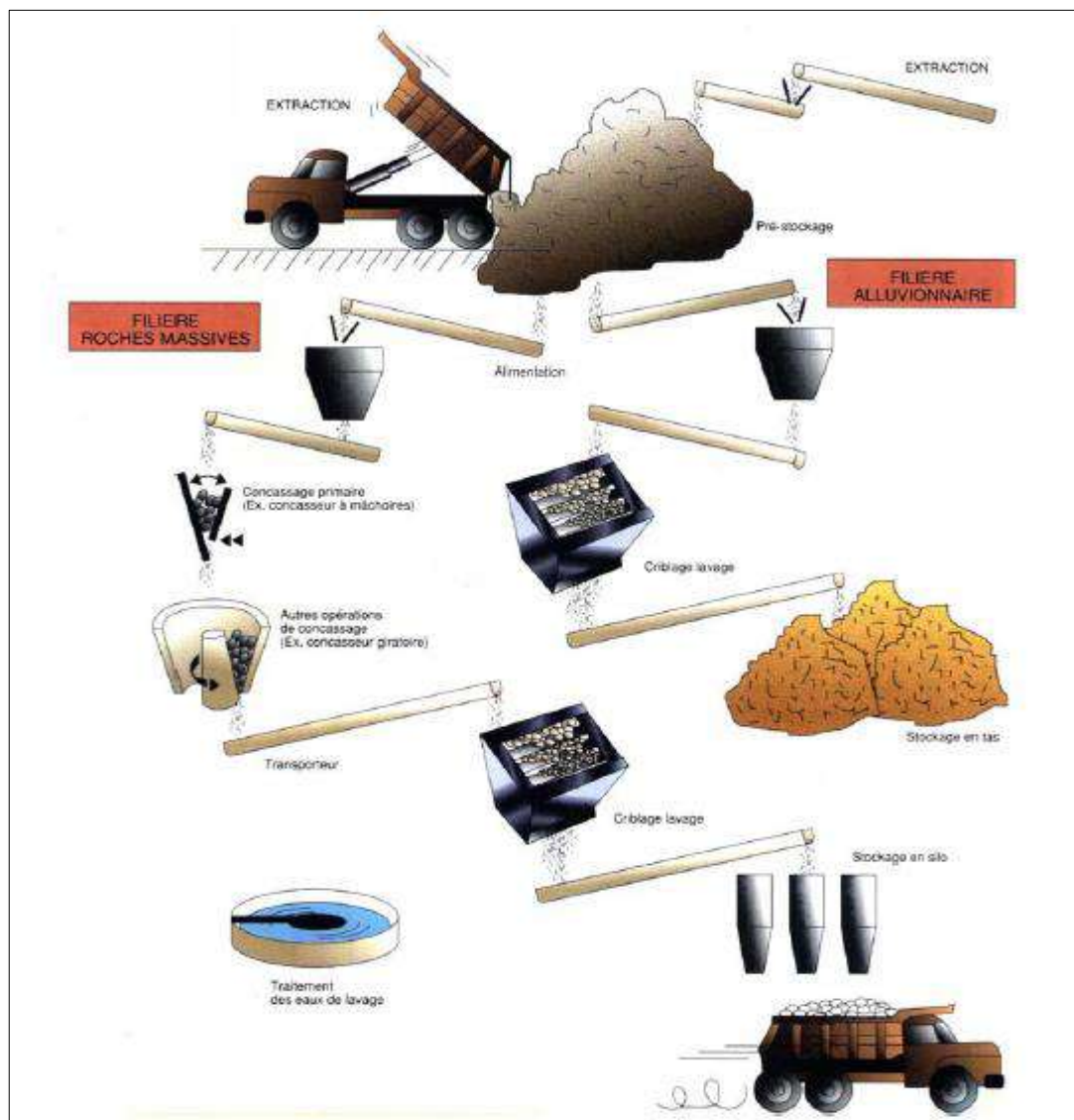
Figure II.6: Extraction des granulats (roches meubles ou massives). (Gabrysiak F., 2013)
