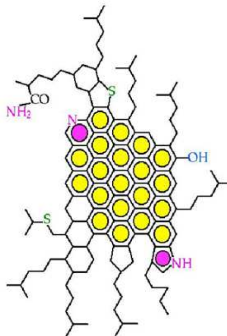
Molecular Structure of Asphaltene Proposed for S10C Residue of Venezuelan Crude by Carbognani [INTEVEP S.A. Tech. Rept., 1992]
