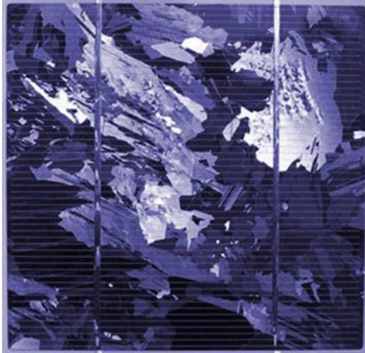
**Figure 1. 3 :** Cellule PV polycristalline
