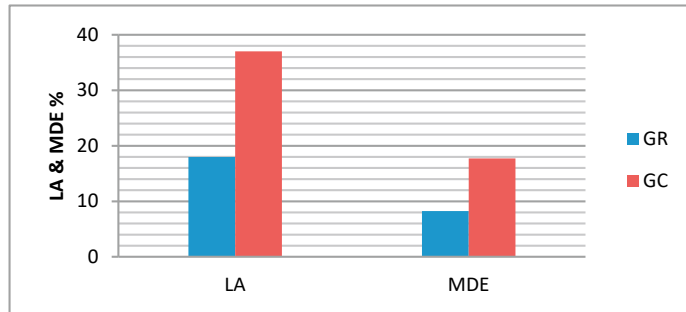
Fig. 3. LA and MDE abrasion resistance results of GR and GC aggregates.
