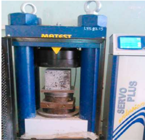
Fig.8. Compressive strength test.
