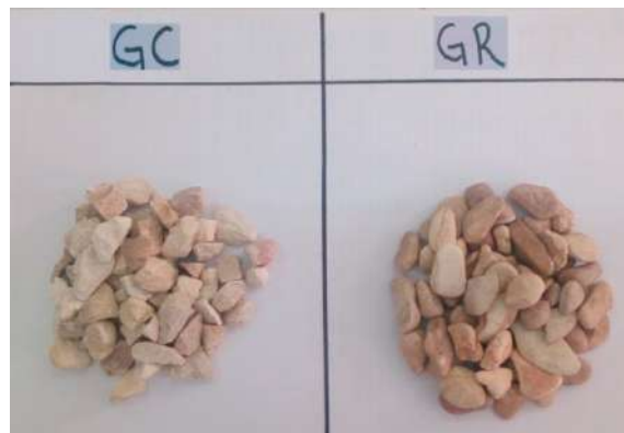
Fig.1. Rounded aggregate (GR) and crushed aggregate (GC).
