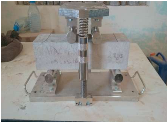
Fig.10. Flexural tensile strength test.
