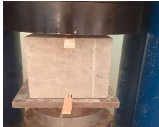
Fig.11. splitting tensile strength test
