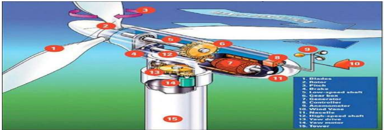
Figure I.5: the component of wind turbine
