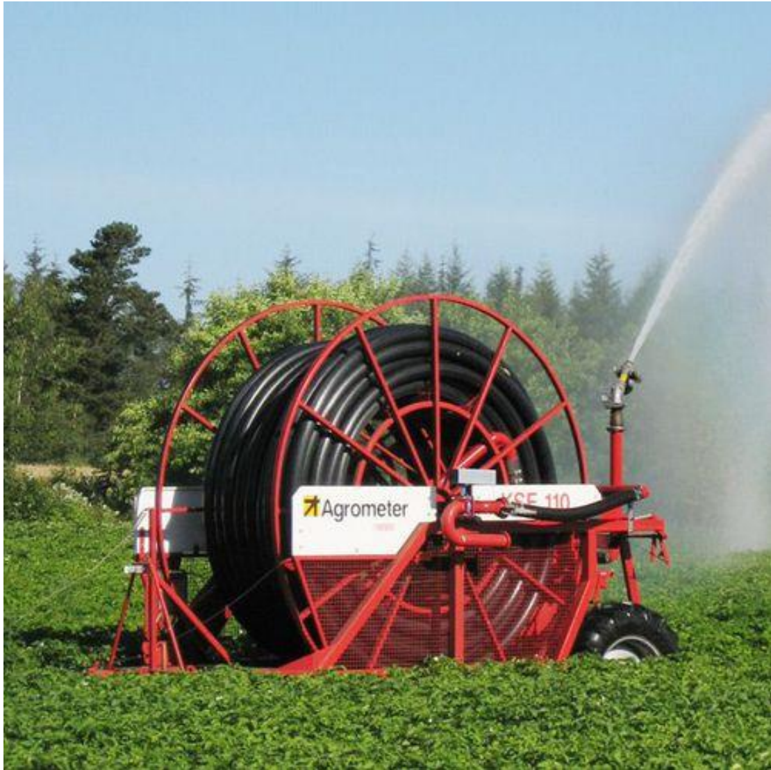
Figure I.12 Arrosage mobile, propulsion
