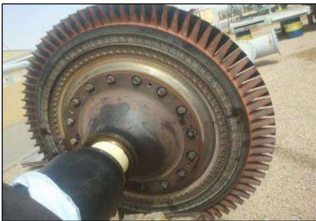
Figure II.27 : Roue de turbine HP
