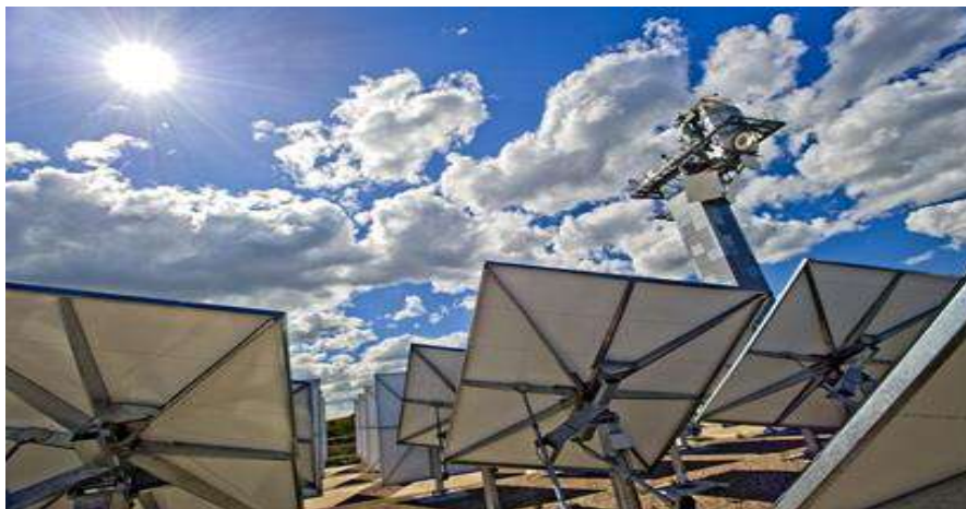
Figure I-18: CSIRO heliostat with single facet and horizontal primary axis which enables the usage of linear actuators for both axes (CSIRO).
