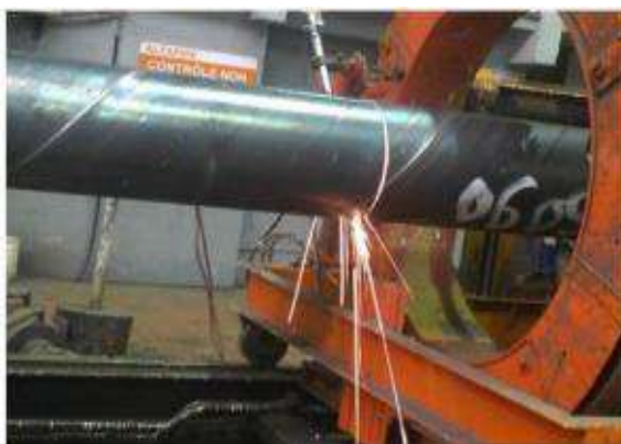
Figure I.17 Processus Oxycoupage de tube
