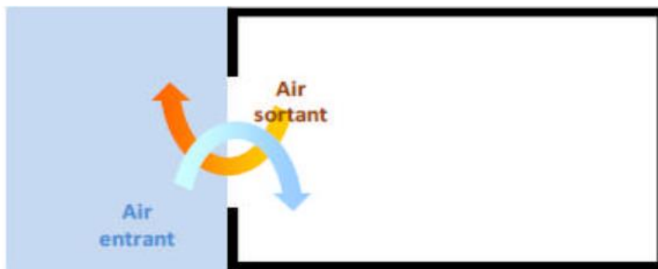
Figure. II.23. La ventilation simple exposition [3]
