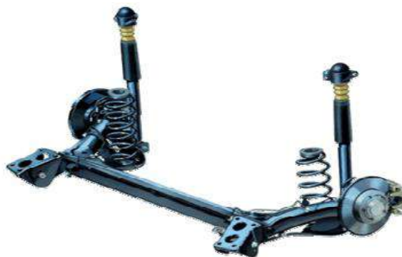
Figure II.10 : Essieu semi rigide de la Golf
