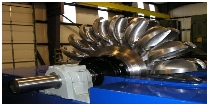
Figure I.2: Pelton wheel turbine
