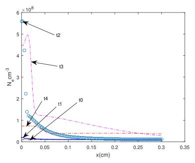
Figure 4.2 – Electron density as a function of distance from the surface.
