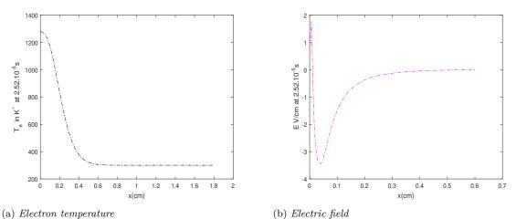
Figure 4.7 – Distributions of electron temperature and electric field as a function of space at the time when surface has a maximum temperature.
