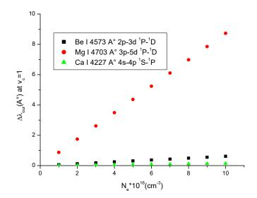
Figure 5.6 – Variation of Stark broadening with electron density at  $v_c = 1$  for Be I, Mg I and Ca I.
