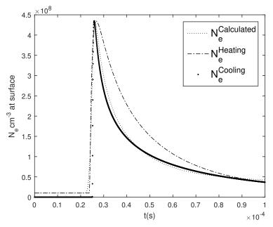
Figure 4.9 – Heating and cooling approximated to numerical calculation of electron density at the surface
