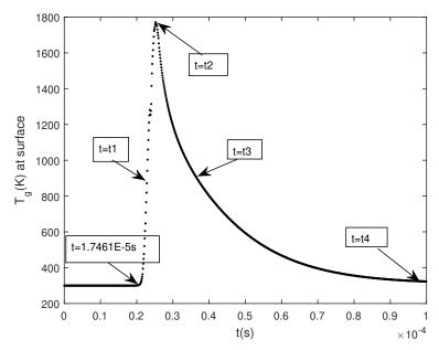
Figure 4.1 – Characteristic times for surface temperature.
