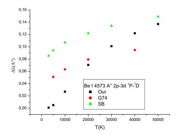
Figure 5.3 – Comparison of Stark broadening at  $N_e = 10^{16} \text{ cm}^{-3}$  with (G74) and SB for Be I.
