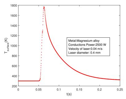
Figure 2.2 – Calculated surface temperature by S. Lemkeddem et al. in (2018).
