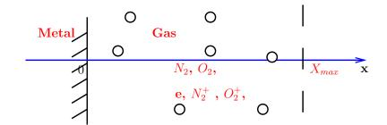
Figure 2.1 – Simplified scheme of  $O_2/N_2$  gas mixture near surface during Laser welding.
