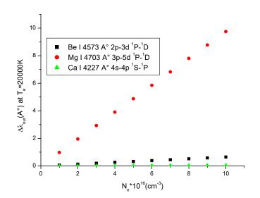
Figure 5.7 – Variation of Stark broadening for Be I, Mg I and Ca I at  $T_e = 20000K$ .
