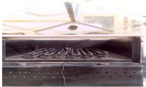
Figure II.2: Emplacement of the heat exchanger inside the drying room.
