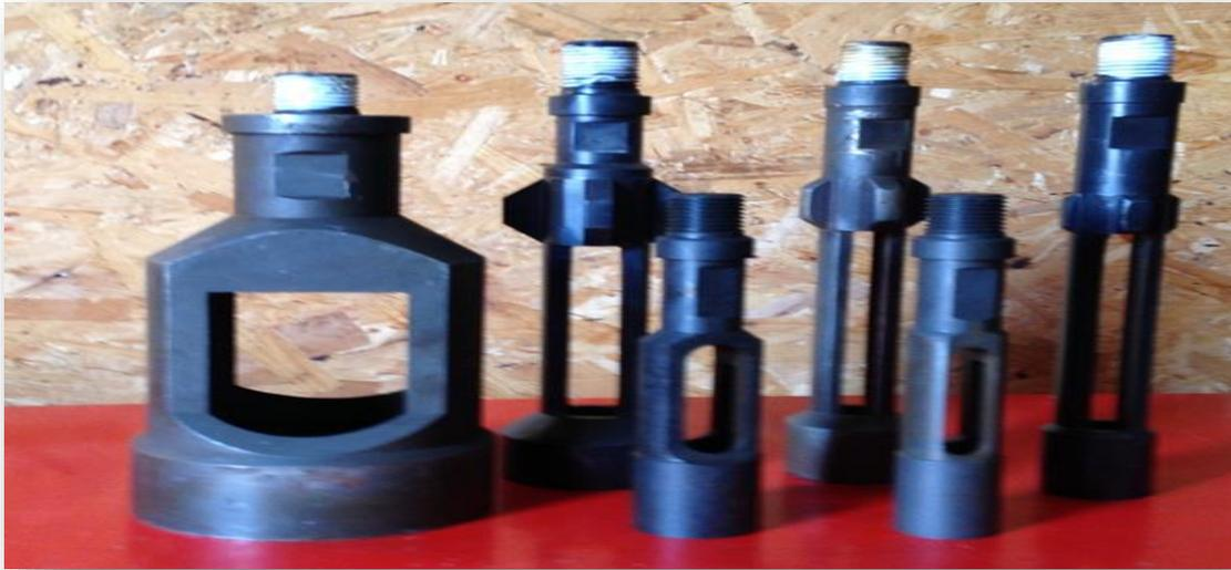
**Fig.III. 10: Gauge Cutter (outil wire line).**
