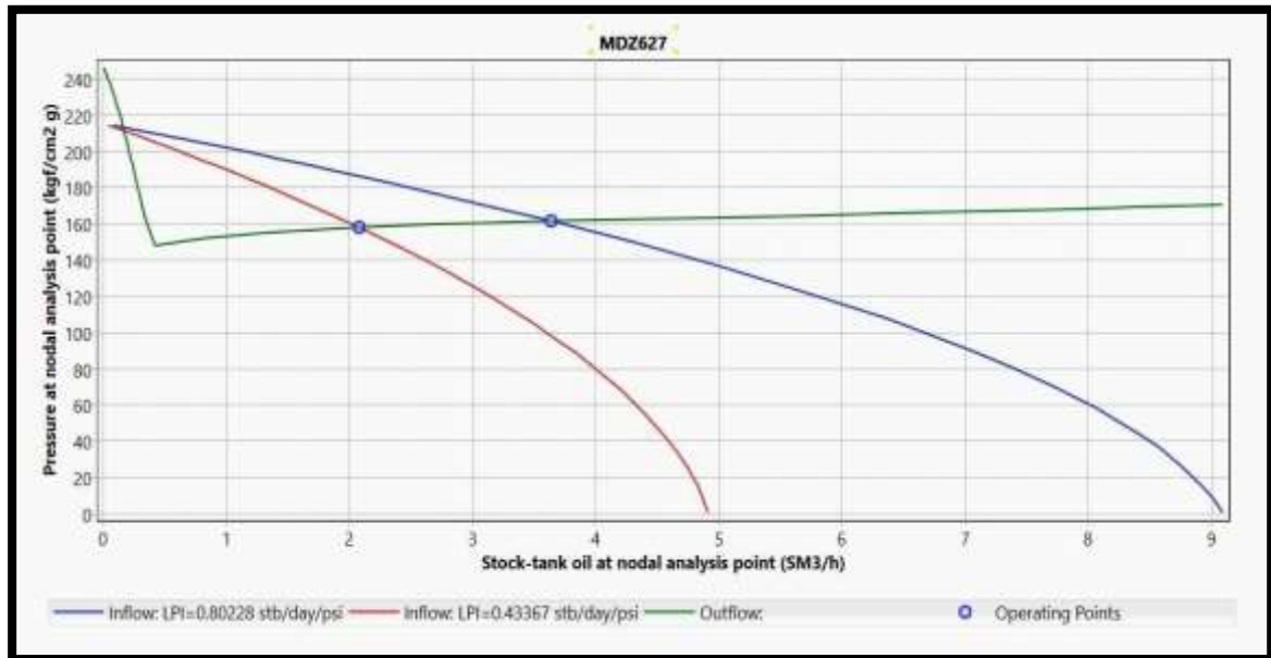
Figure IV.12: the operating point of well MDZ627 before and after the descent of the semiintelligent completion
