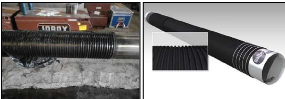
Figure III. 3: Real photo of the rubber part of the Casing Patch [13].
