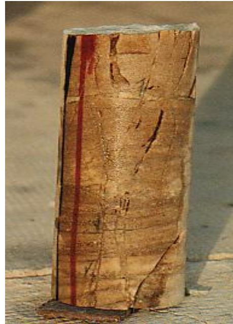
Figure IV.3: Typical Lower Zone Shear Fractures.[24]
