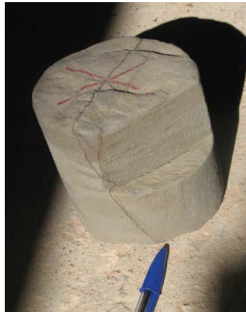
Figure IV.9: Example of a fracture present in a core extracted from a production well in Krechba.
