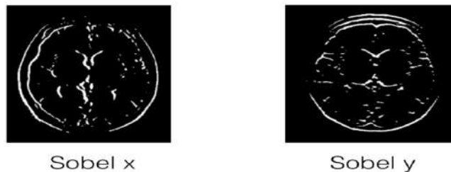
Fig14. Sobel x and y filters (left and right) applied to an image of a brain [XXX]
