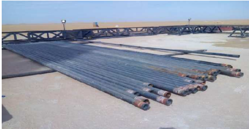
Figure II.4: tubing de production
